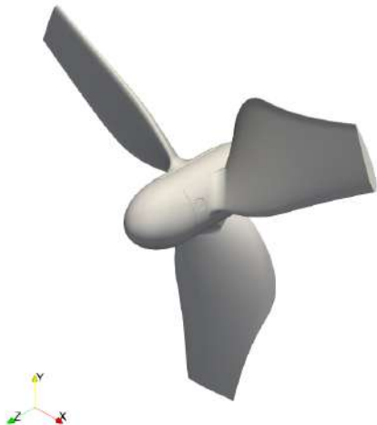
Cleaned rotor geometry as STL
